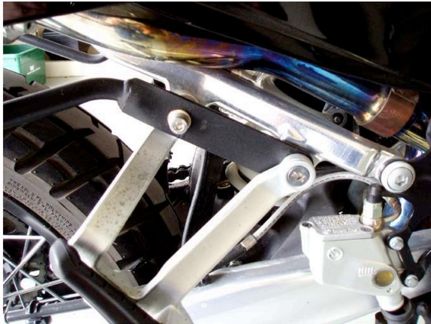
Reinstall right side passenger foot peg bracket as shown. Install supplied 8x30mm flathead screw in forward position with mount support between bike subframe and bracket. Install 8x60mm cap bolt in rear position in following order. 1) Install 8mm bolt through mount support, 2) install ¼" spacer between mount support and foot peg bracket, 3) install 8mm washer between foot peg bracket and bike subframe.
