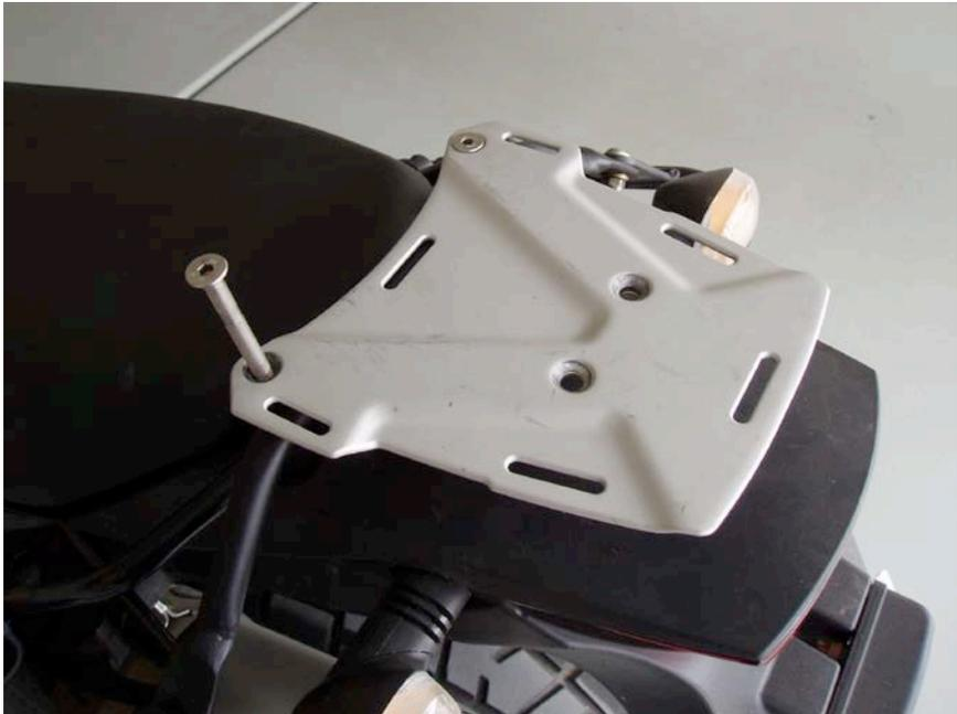
forward bolts with the supplied 8x90mm flathead bolts as shown. Replace the stock 2 rear bolts with the supplied 8x60mm flathead bolts, using the 2 supplied 1” spacers between the rear rack and grab bar.
