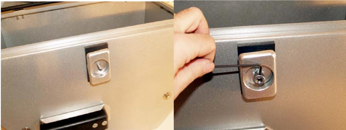
Peel off the protective covers on the composite block tape strips, place over the hole in the bag as shown. Push the crank handle shaft through the hole and thread on the cam. Add the supplied washer next. Use the supplied Allen to tighten the setscrew, ensuring the setscrew is seated into the indentation. Repeat on the other side bag. Keep the lower mounting plates loose for now.
