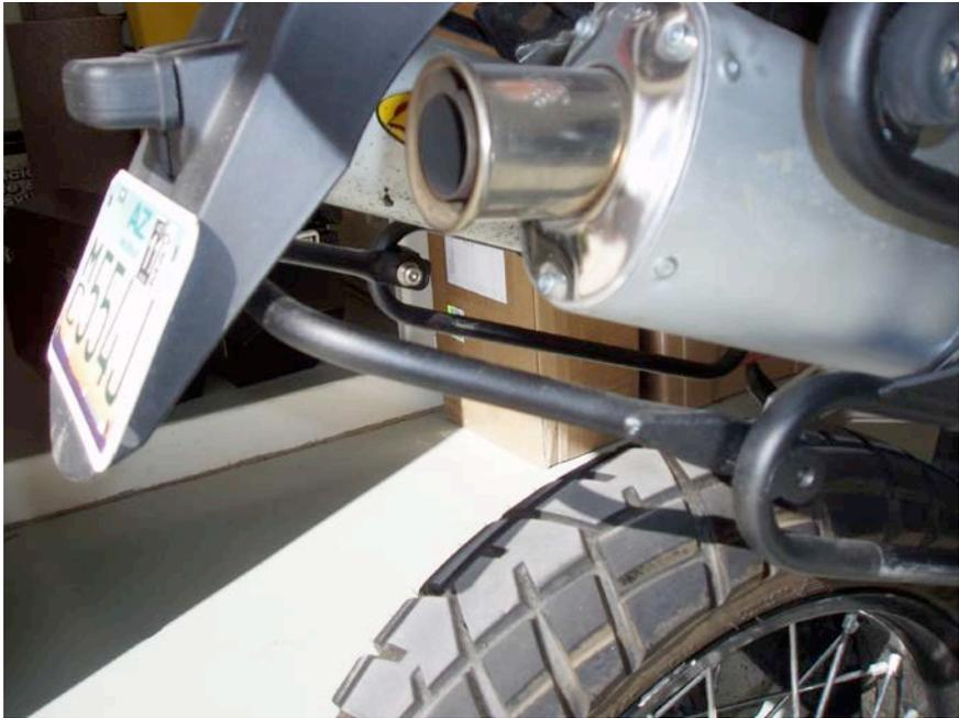
Install lower rear mount support using supplied 8x50mm flathead bolts, washers and nylock nuts.
