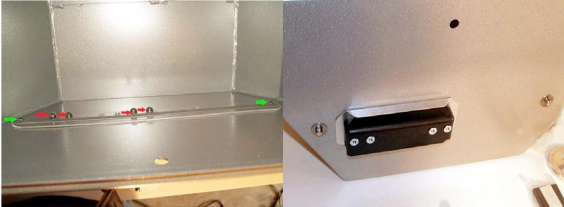
washer and through the bag into the metal plate and threaded composite block (right). Keep these loose for now.
