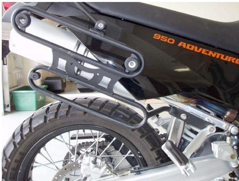
Repeat steps for right side main mount, starting with removing stock grab bar bolt, and installing mount using supplied 8x80mm cap bolt.
