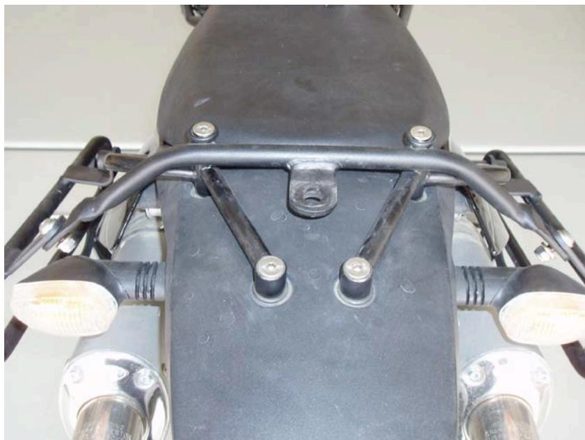
Remove stock grab bar bolts. Install rear mount support as shown, replacing the stock bolts with supplied 8x90mm flathead bolts. Connect rear support to right and left main mounts with supplied 8x25mm button head bolts, washers and nylock nuts. If using stock rear rack, see below.
