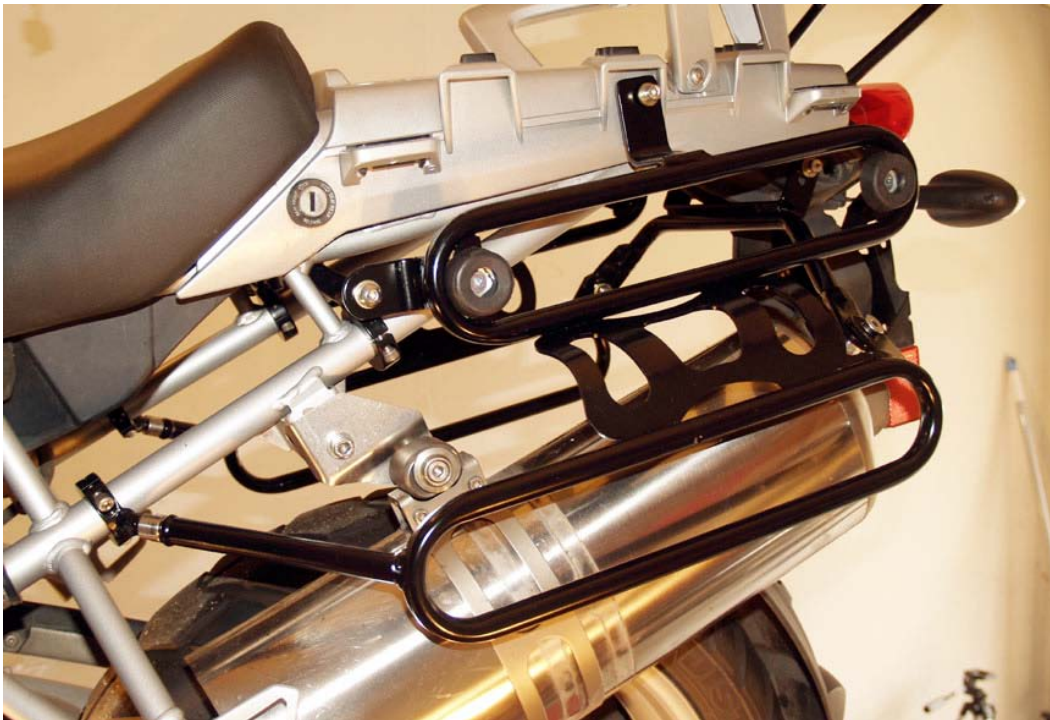
Brackets installed, high muffler mount shown, low muffler mount similar.
