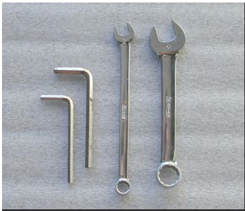
Figure 1 Tools Required – 5mm, 6mm allen and 10mm, 13mm wrench, plus a drill with 6mm or 1/4” bit
